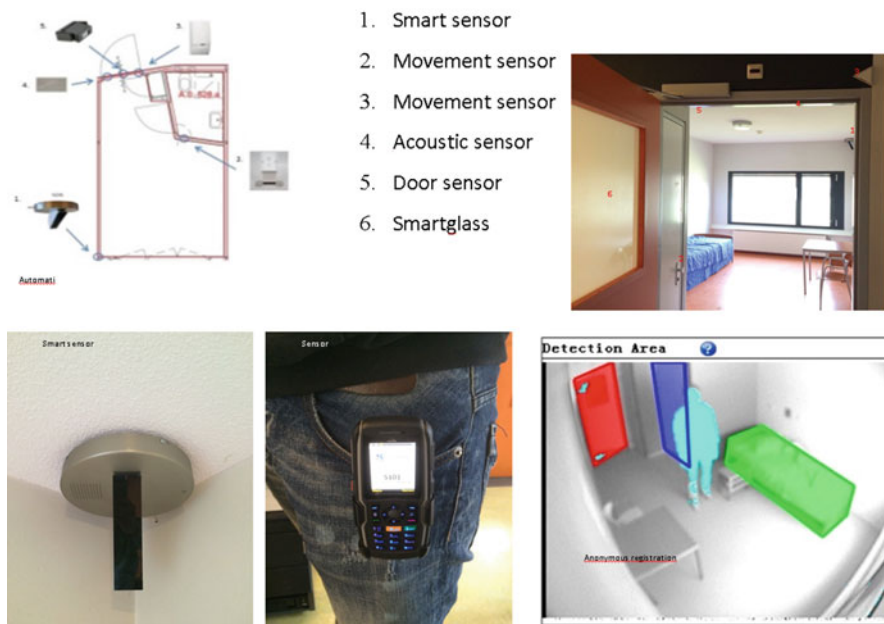
Picture 1 Technical details for the automation room
